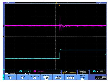
Figure C.3 – 0.5 meter cable displaying cross-talk
