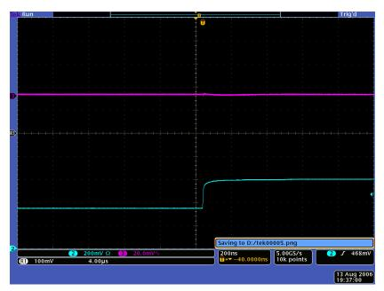
Figure C.4 – 20 meter cable displaying no cross-talk
