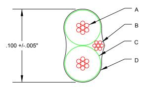
Figure 2.1 Single Twisted Pair Assembly
