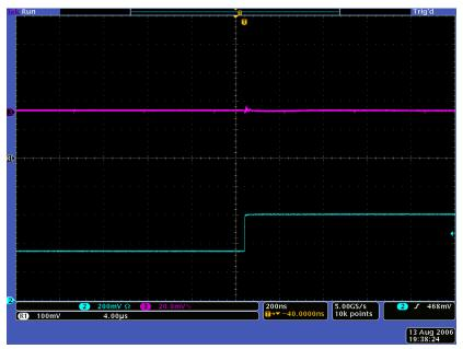
Figure C.2 – 0.5 meter cable displaying no cross-talk
