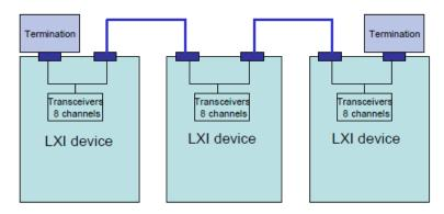
Figure 1.1 Configuration of LXI Devices using the LXI Wired Trigger Bus
