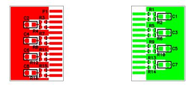
Figure 4.3 Example termination pads
